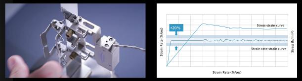
Strain rate control, in which the rate of deformation measured by an extensometer is controlled to be constant, requires highly accurate control to follow rapid changes in material behavior. Metal Tensile Test Standard: ISO 6892 (JIS Z 2241) specifies that the allowable range of increase in strain to the yield point is  $\pm$  20% or less. The strain rate control specified in ISO 6892 (JIS Z 2241) is possible<sup>\*1</sup> to achieve with the AGX-V for many materials.
