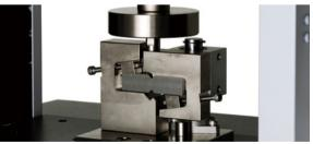
Open Hole Compression Test Jig (OHC Test, ASTM D6484) This is a compression test jig for an open hole test sample that has a circular hole in the center.
