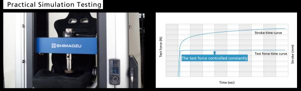
To maintain engine mounts and other rubber materials at a constant test force, it is necessary to gradually change the retention position to suit the characteristics of the test sample. In order to maintain the test force at a constant value, high control stability is required, with high control responsiveness and no vibrations generated due to excessive response.\*<sup>2</sup>
