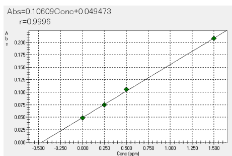
Fig. 3 Calibration Curve of Fe
