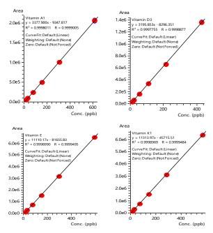
Fig. 3 MRM calibration curves of vitamin A1, D3, E, and K1 in the range of  $10{\sim}600$  ng/mL .
